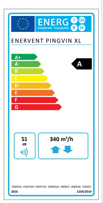
The information on the energy label for this product has been defined with local demand control. Local demand control means that the ventilation unit continuously regulates the fan speed(s) and flow rates based on more than one sensor. Please remember to connect all local senseors (some sold as extra equipment) in order to accieve the declared energy class.
