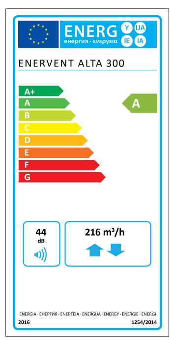
The information on the energy label for this product has been defined with local demand control. Local demand control means that the ventilation unit continuously regulates the fan speed(s) and flow rates based on more than one sensor. Please remember to connect all local senseors (some sold as extra equipment) in order to accieve the declared energy
