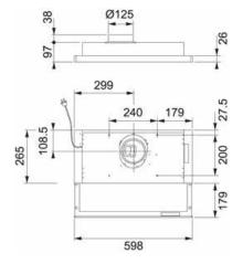
This premium cooker hood is designed to be embedded in the furniture. The electronic switches are in the pull-out front. This model has an electrically closing damper and indication signal to the unit. The color options for the front list are white and stainless steel.
