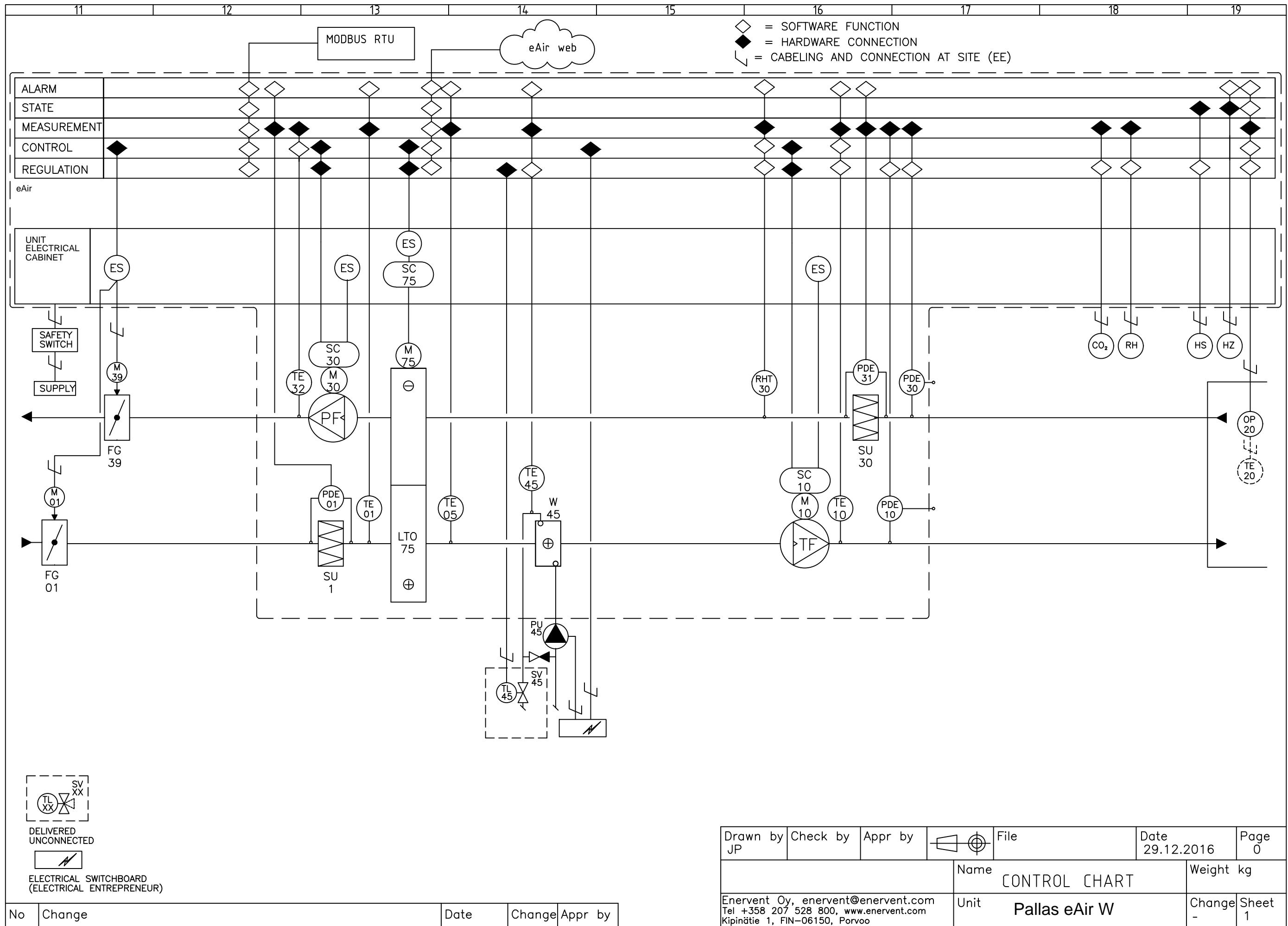
Filter change guards and Constant duct pressure regulation can be added or removed from the schematic by turning the layer ON or OFF
