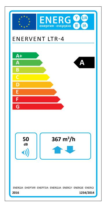
The information on the energy label for this product has been defined with local demand control. Local demand control means that the ventilation unit continuously regulates the fan speed(s) and flow rates based on more than one sensor. Please remember to connect all local senseors (some sold as extra equipment) in order to accieve the declared energy
