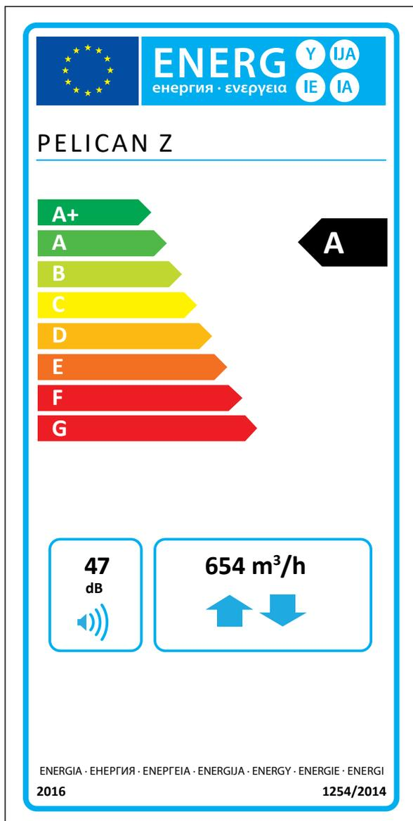
The information on the energy label for this product has been defined with local demand control. Local demand control means that the ventilation unit continuously regulates the fan speed(s) and flow rates based on more than one sensor. Please remember to connect all local sensors (some sold as extra equipment) in order to achieve the declared energy class.
