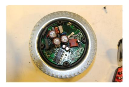
The disassembly method for the fan of the Pallas device is different. Remove the fan cover and detach the wires. Dismantle the fan until you locate the circuit board. Deliver the circuit board for WEEE recycling. Other fan components are metal waste.
