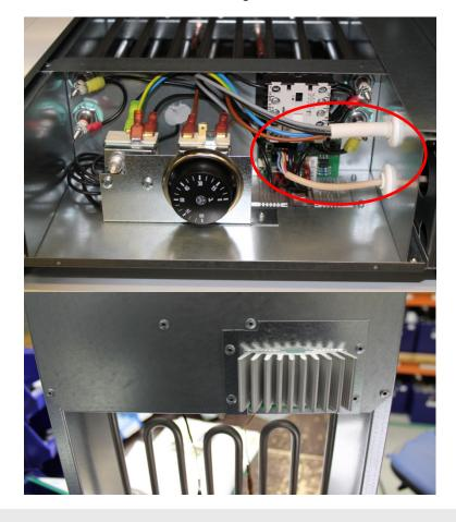
For the electric coil of the Pallas device, the components inside the red circle must be delivered for WEEE recycling. Other components can be delivered for metal waste recycling.
