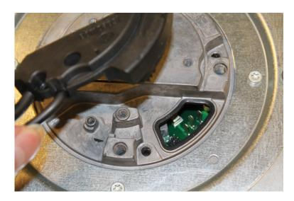
Lift the fan out of the chamber.
