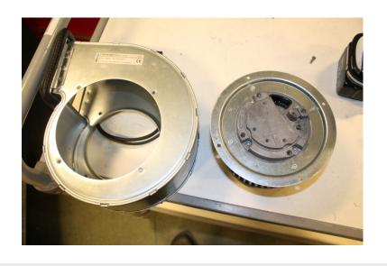
The alternating-current fans can be delivered for metal waste recycling without disassembling them. The alternating-current fans can be identified on the condenser which is located in either the electrical cabinet or the fan. The condenser must be delivered for WEEE recycling.
