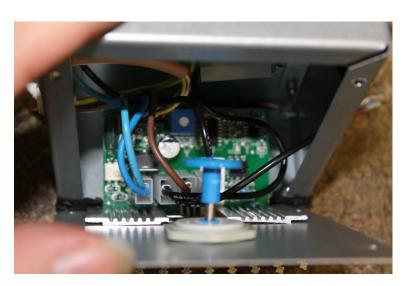
The circuit board must be delivered for WEEE recycling.
