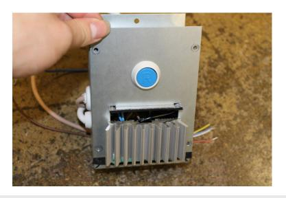
The electric coil of the Pandion, Pelican and Pegasos devices must be removed from the unit first. Next, open the four screws in the cover, using a flat-head screwdriver or an open-end wrench. Pull the cover off. Detach all wires from the circuit board.
