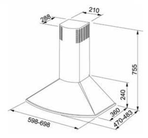
Scandinavia's most popular hood. This model is installed on the wall. The Franke Tender hood has an activated carbon filter and indication signal to the unit.
