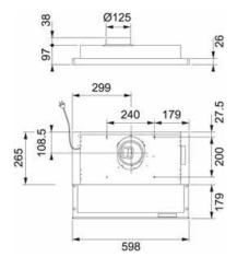
This premium cooker hood is designed to be embedded in the furniture. The electronic switches are in the pull-out front. This model has an electrically closing damper and indication signal to the unit. The color options for the front list are white and stainless steel.
