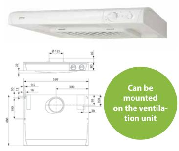
This is a popular basic cooker hood. This model has closing damper with timer and indication signal to the ventilation unit (closing contact). The ventilation unit can be physically connected to this hood.
