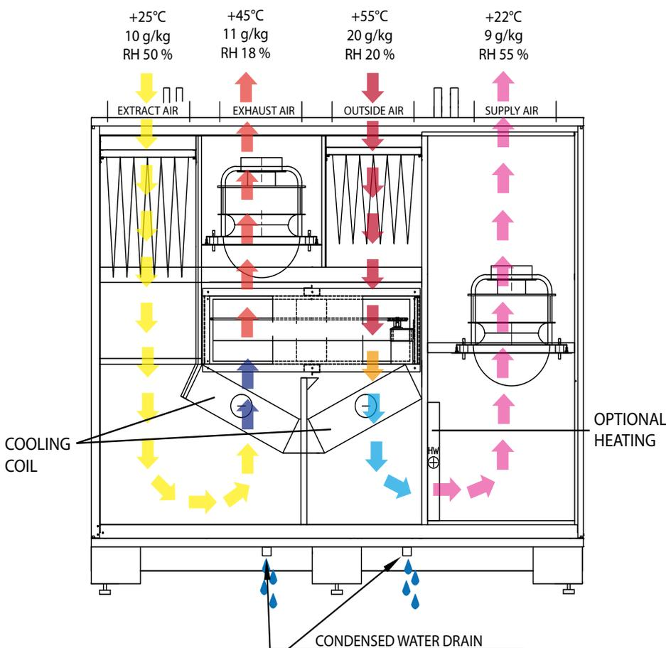
Enervert Pallas Twincoil principle of operation
