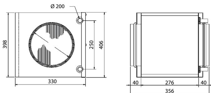
The optional hydronic heating for Pandion twincoil is realized with a duct coil
