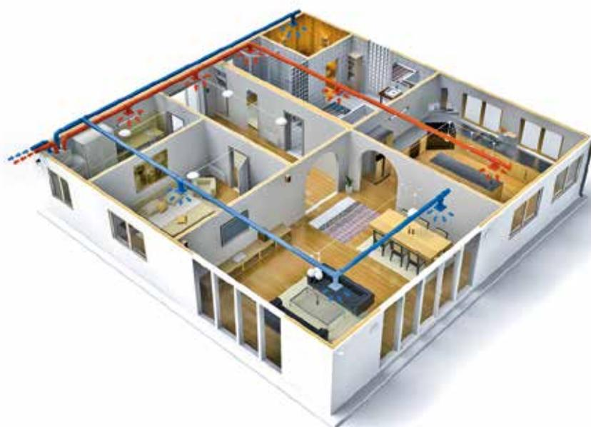
An example of a mechanical ventilation system. The blue ducts show the path of the fresh, filtered and cooled/dehumidified or warmed incoming replacement air. The red ducts show the path of the stale extract air.
