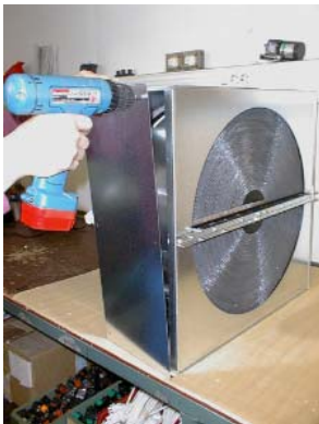
Picture 1 : removal of cover, 6 screws Picture 2 : loosening of space beam
