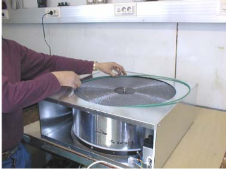
Picture 3 : inserting the new belt
