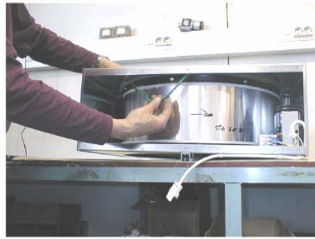
Picture 4 : pulling through the new belt.
