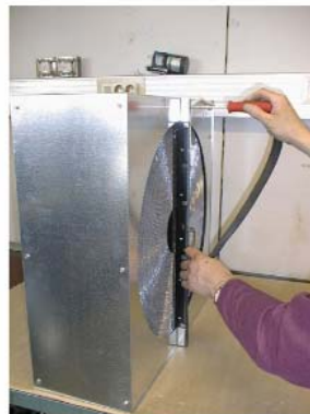
Picture 1 : removal of cover, 6 screws Picture 2 : loosening of space beam
