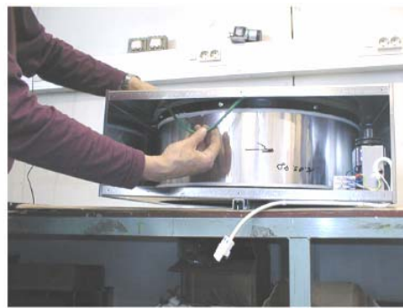
Picture 4 : pulling through the new belt.
