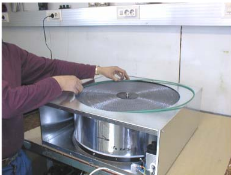
Picture 3 : inserting the new belt
