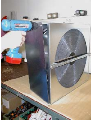
Picture 1 : removal of cover, 6 screws
