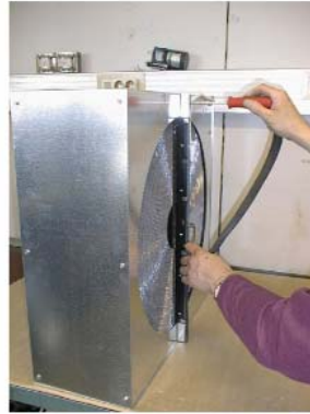
Picture 2 : loosening of space beam
